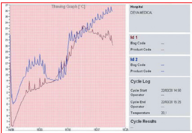
Figure 2: To thaw one or more 600 ml bags , cycle time can be set between 25 and 27 minutes, with tray temperature of 40°C.
