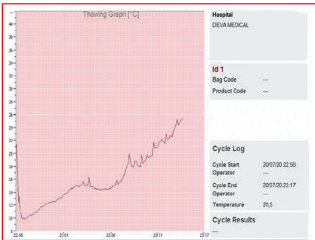
Figure 1: To thaw one 260 ml bag , cycle time can be set between 15 and 18 minutes with tray temperature of 40°C.
